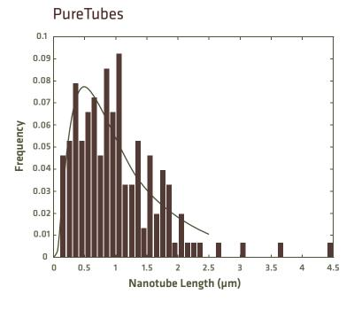
**Figure 6.** Atomic-force microscopy (AFM) data indicates that our SWNTs range in length from approximately 100 nm to 4 microns. **A. B. C.** Length histograms of our IsoNanotubes-M, IsoNanotubes-S, and PureTubes, respectively.
